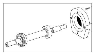
H. Shaft Assembly Removed.
